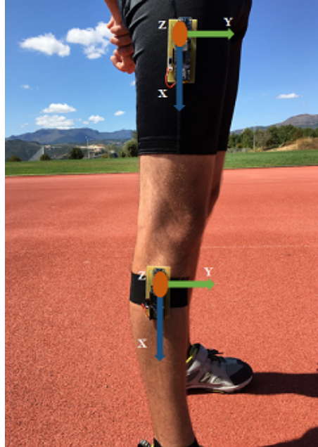
Figure 5.3: Anatomical placement of the devices, lateral configuration.
