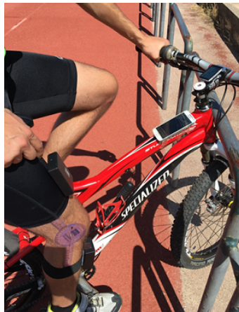
Figure 5.1: Smartphone position on the bicycle.
