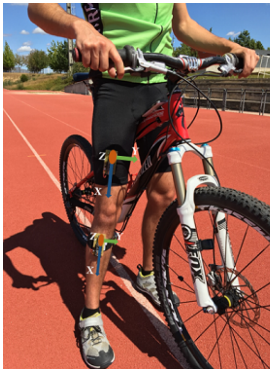
Figure 5.7: Anatomical placement of the devices, frontal configuration.
