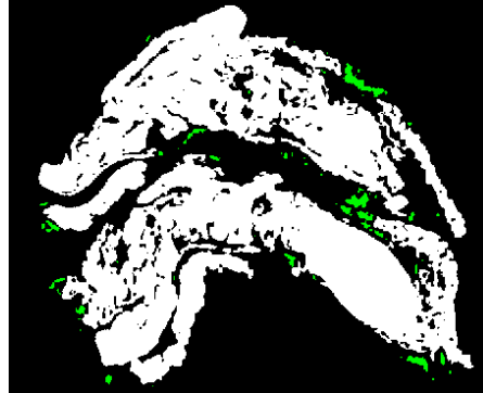
Figure 3. Identification of the regions (in green) to be discarded from an experimental image.
