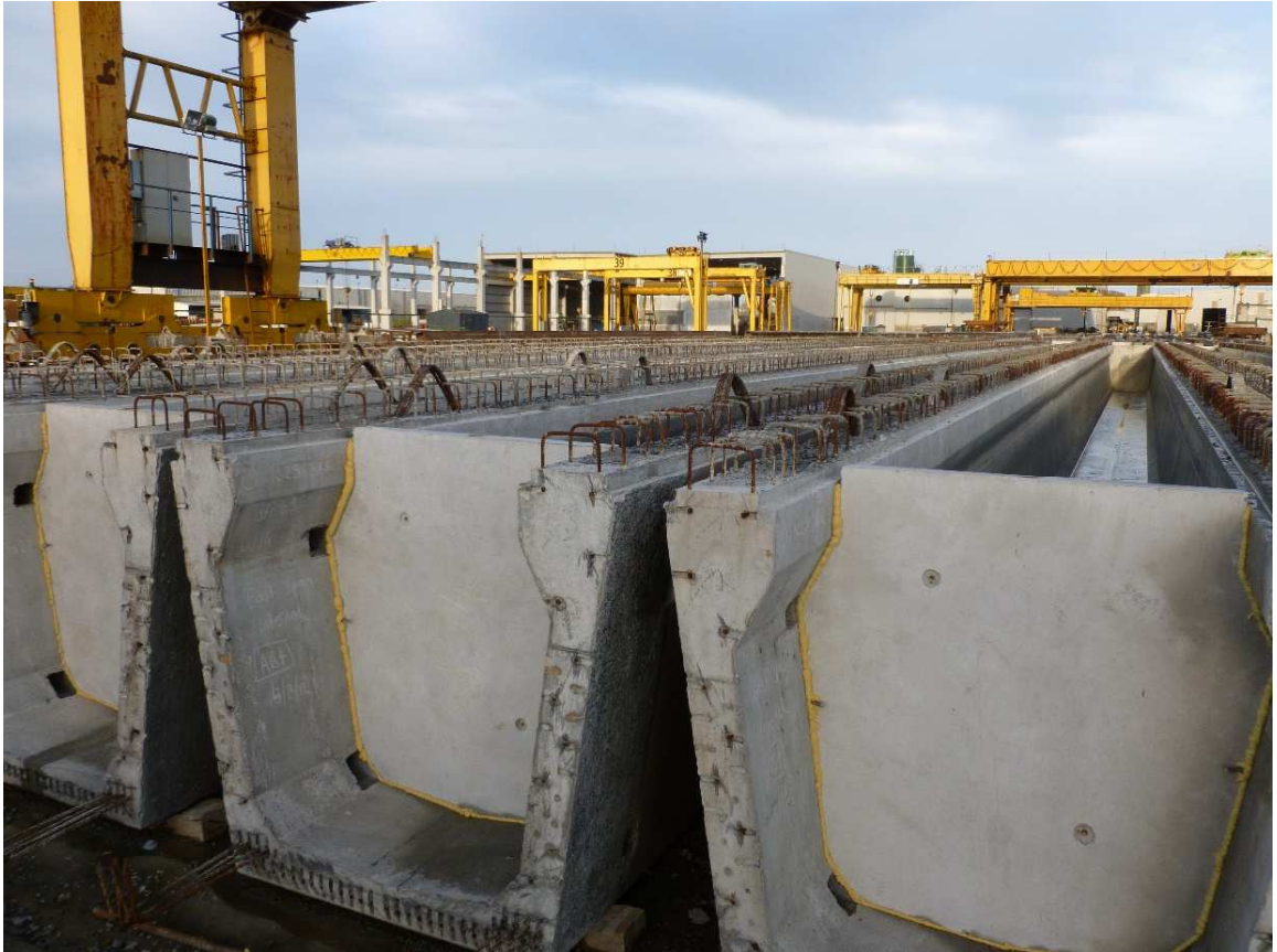
Figure 1-3 – Precast U-shaped beams for bridge decks (Banagher 2015).
