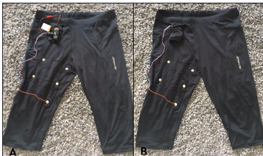
Figure 4.9 - Conductive wearable shorts used for EMG signal collection. A) Illustration of the electrical components. B) Illustration of the electrical components stored in a pocket.
