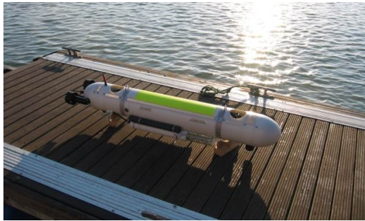
(a) MARES AUV configured for a rapid environmental assessment mission.
