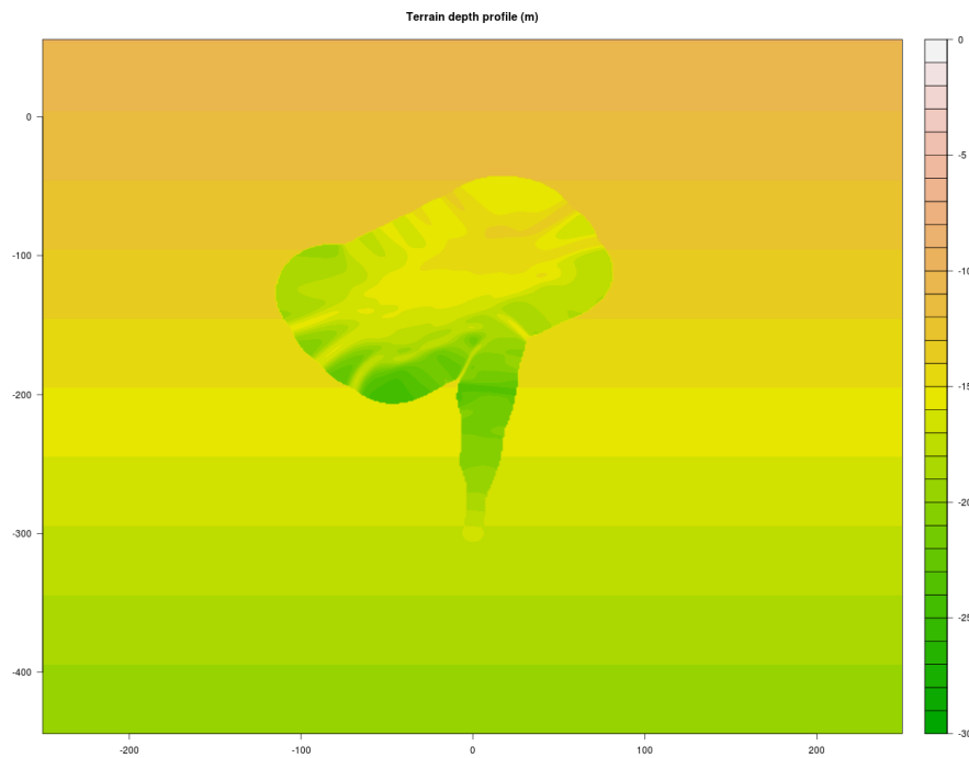
(c) Resulting DEM after combining a local map from a vehicle. The smoothness of the elevation measurements here is closely related to the variance of the elevation measurements on the original map.
