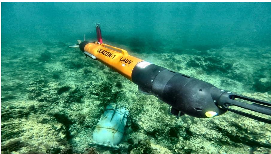
Figure 1.2: A typical Autonomous Underwater Vehicle. Source - LSTS
