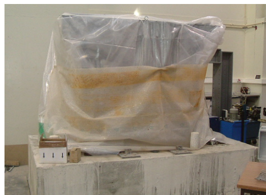
Fig. 22. Simulation of local air moisture conditions.
