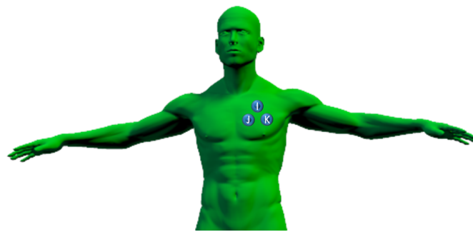
Figure 4.3: Chest electrode placement used for ECG acquisition
