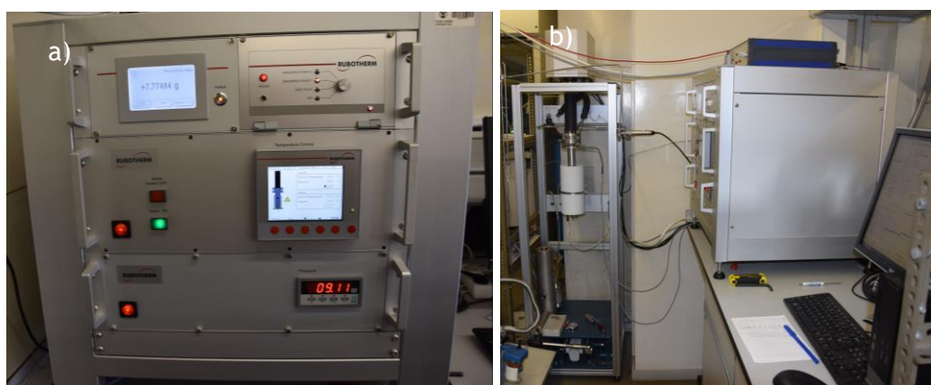
Figure 4- a) Magnetic suspension microbalance (Rubotherm, Germany); b) Acquisition system of the magnetic microbalance.
