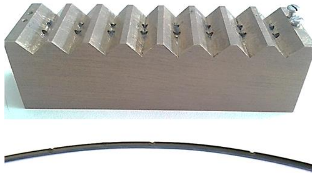
Figure 14. Brass mold employed to create the grooves in the POF, below the mold a detail of the POF with the grooves is shown.
