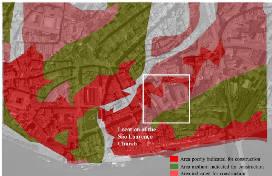
Figure 43. Mapping of soil classification for construction according with Porto Geotechnical Report and location of the São Lourenço Church.
