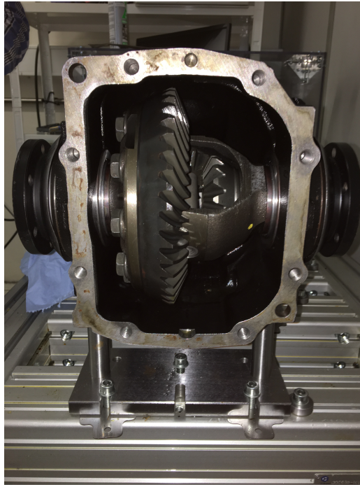
Figure 5.2.: Differential Under Study.
