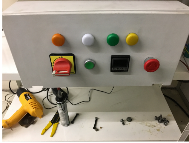
Figure 5.5.: Temperature Control Panel.
