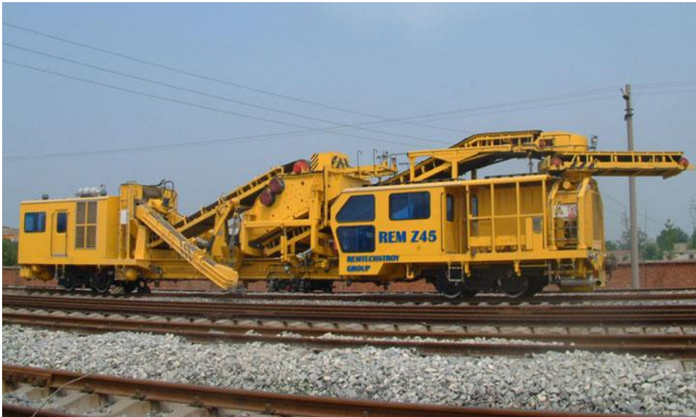
Figure 2.15 – Ballast Cleaning Machine [Remtech, 2010]
