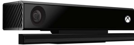
Figure 2.11: Structured Light camera Kinect v2 from Microsoft.
