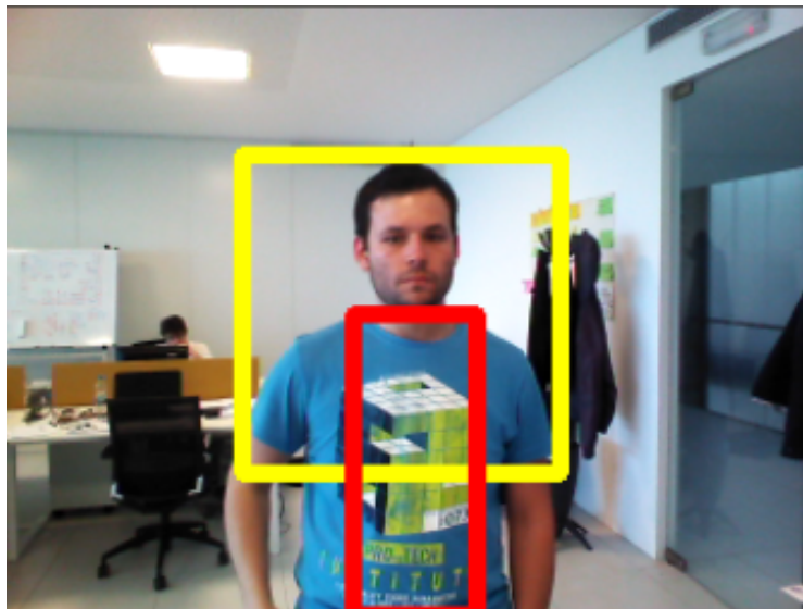
Figure 4.6: RGB image representing with a yellow square the identification from the robot, identification and with the red square the region of interest to calculate the threshold value.
