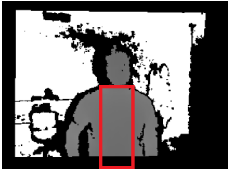
Figure 4.7: Depth image correspondent to the image 4.6 with the red square representing the region of interest of depth values that will be used to calculate the threshold value to use in further operations.
