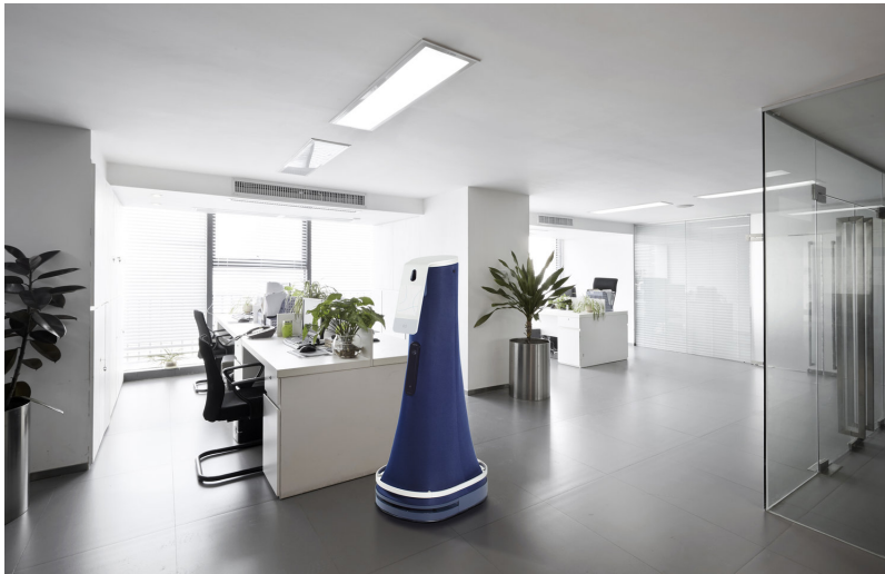
Figure 2.5: Robot from Cobalt Robotics performing the surveillance of an office [7].
