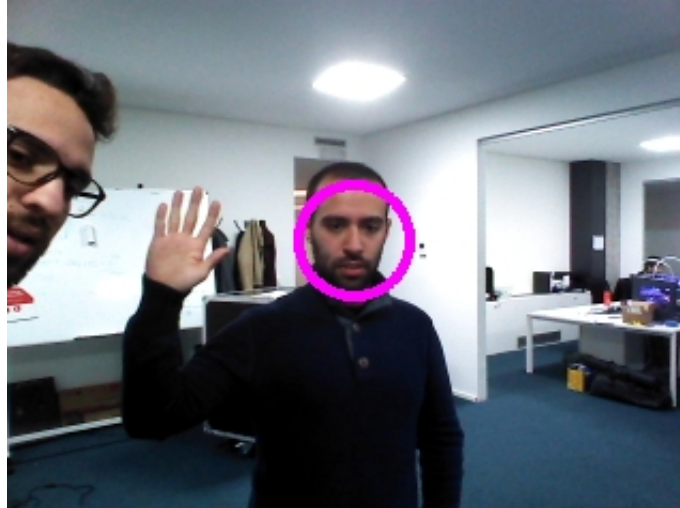
Figure 4.5: RGB image received from the robot with the face detection of the user.
