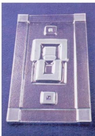
Fig. 17. Example of one part obtained with one mould of ceramic fibres.
