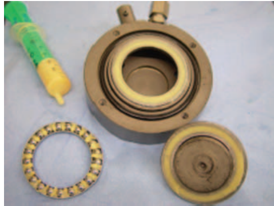
Figure 2. Grease lubrication of the thrust rolling bearing.
