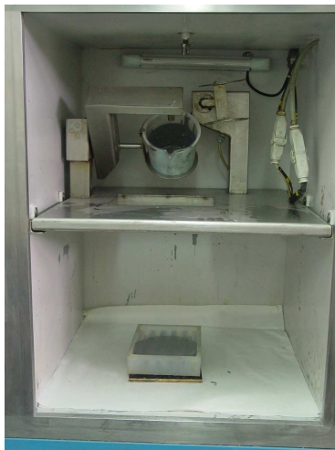
Fig. 5. Vacuum equipment is an indispensable tool to control the porosity level in resin composites.
