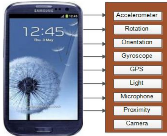
Figure 3.4- Various embedded sensors in modern phone - e.g. Galaxy S4 phone representative of numerous sophisticated mobile devices with a growing number of embedded sensors
