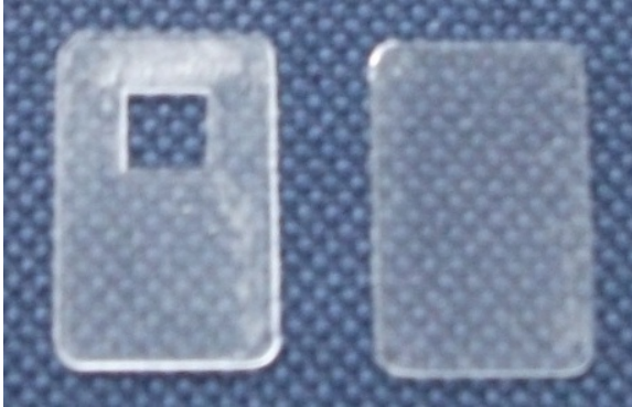
Fig. 3. Molds made of polydimethylsiloxane (PDMS)
