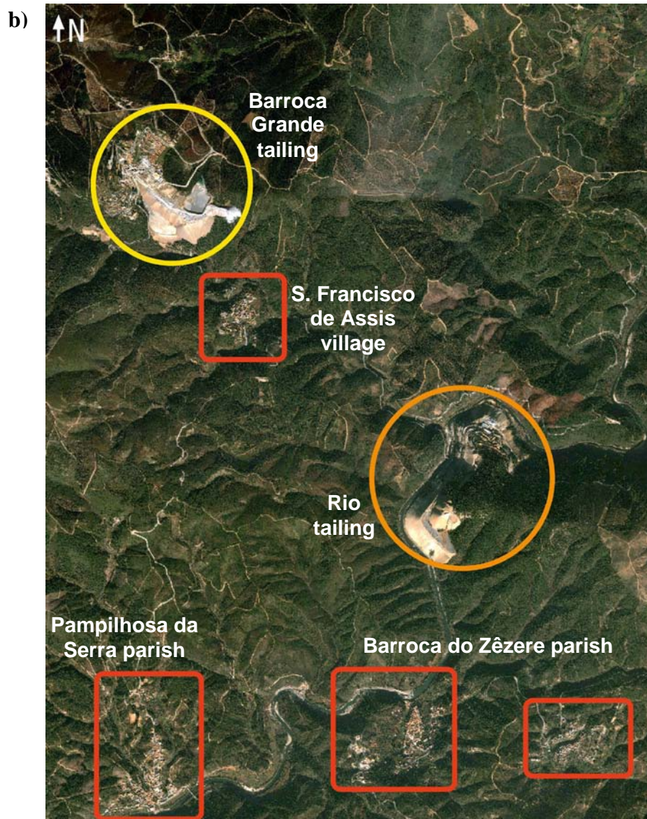
FIGURE 1 – (a) Location of Panasqueira mine (red arrow on the left map), the Castelo do Bode dam, and the Zêzere river flow (blue line across the map on the right); (b) Map showing the location of Rio tailing ( \sim 1,200,000\text{m}^3 ) and mud impoundment ( \sim 731,034\text{m}^3 ) (orange circle), Barroca Grande tailing ( \sim 7,000,000\text{m}^3 ) and two mud impoundments ( \sim 1,193,885\text{m}^3 ) (yellow circle) and several small villages nearby these structures (red squares: the one in the upper left corner is S. Francisco de Assis; the other three on the bottom belong to Barroca do Zêzere and Pampilhosa da Serra parishes). One can also see Zêzere river flowing from the middle right side, close to Rio tailings where it merges with a small river (Casinhas creek) coming from upstream Barroca Grande and that passes through S. Francisco de Assis, and then flows down nearby the villages from Barroca do Zêzere and Pampilhosa da Serra parish. Image adapted from Candeias (2010).
