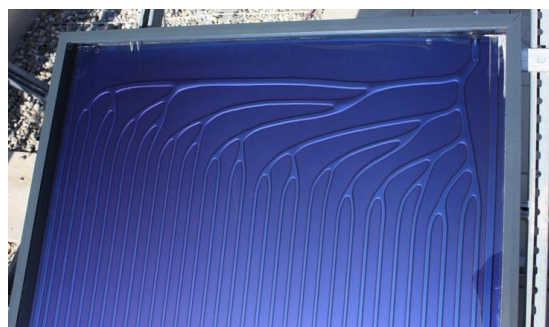
Figure 2.14 - First generation BIONICOL prototype collector (© Fraunhofer ISE) (ISE, 2015)
