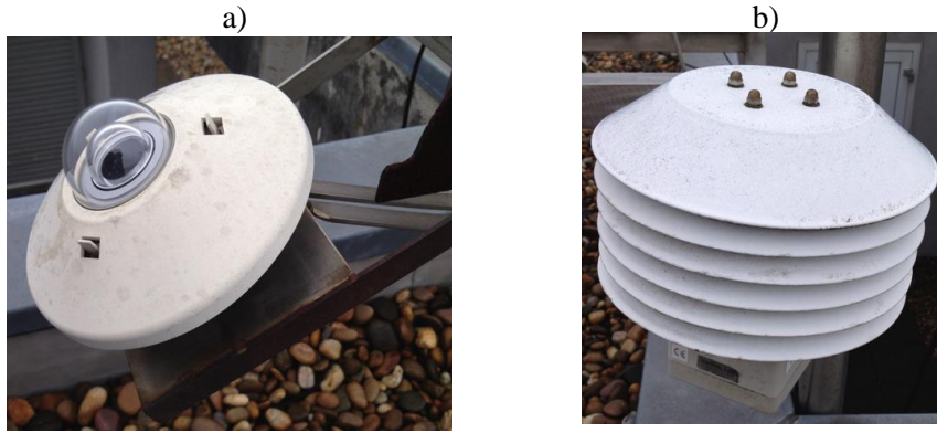
Figure 3.4 - Sensors used in the measurements a) Pyranometer b) Temperature and humidity sensor
