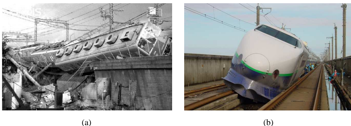
Figure 1.3 - Train derailments on bridges: (a) derailment during the Kobe Earthquake (CorbisImages, 2014) and (b) derailment during the Mid-Niigata Earthquake (Ashford and Kawamata, 2006)
