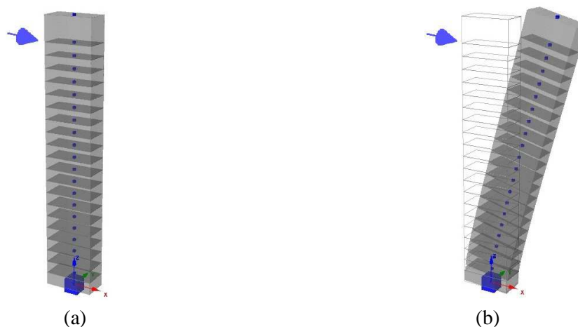
Figure 6.13 - Single degree of freedom model of the pier developed in SeismoStruct: (a) initial position and (b) ultimate capacity deflection (5× amplified).
