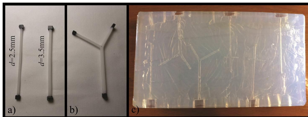
Figure 2.3. Epoxy resin mold made by stereolithography of: a) two straight channels, b) bifurcated channel and c) non-transparent silicone mold containing the various geometries.
