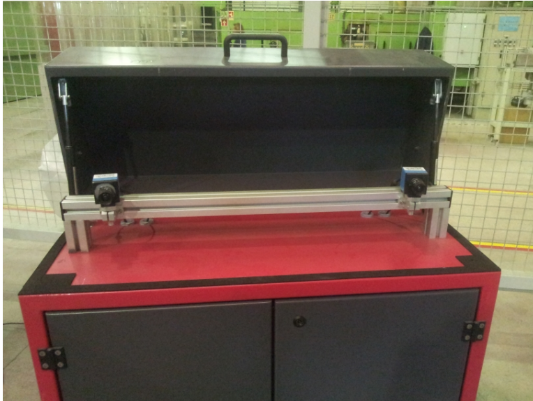
Figure 5.4: Two Camera Arrangement for Stereoscopy - The figure shows the cabinet that holds both cameras. These are separated by 70mm and slightly rotated towards each other. The cabinet has the function of maintaining the cameras' positioning and protect them from dust.
