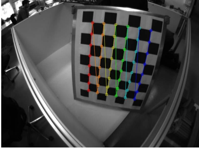
Figure 3.7: Calibration Pattern - A checker-board pattern used for camera calibration. It is the most used method as it simply involves printing a known-size black and white squared pattern. The required image processing is also minimal — finding the black-to-white transitions and detect the corner.
