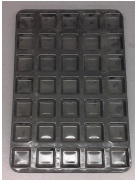
Figure 5.10: A Baking Tray - One of the work pieces coated at Flupol. The discussion on the trajectory features for the remaining of this section is based on the painting path for this shape.
