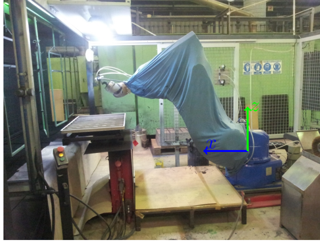
Figure 5.2: Robot in Flupol Coating Cell - This figure shows the work area with the robot operating over a baking tray held by the turn-table. The manipulator occupies the same place and the human did for demonstration (Figure 5.1).
