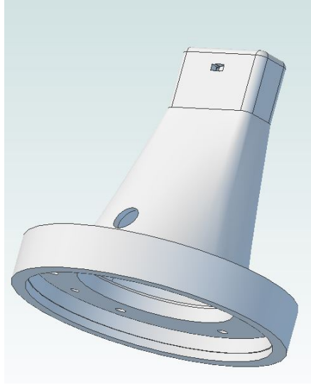
Figure 5.5: CAD Model of the Calibration Tool - This object is attached to the robot end-effector and holds a single LED near the tip. This LED is turned ON at each node of the calibration grid and allows capturing a pair of images corresponding to the node position in space.
