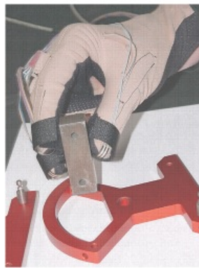
Figure 2.2: Glove - A glove with tactile sensors proposed by Dillman, R et al [33]
