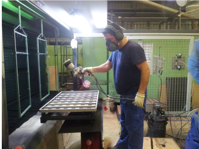
Figure 5.1: Human Painter in Flupol Coating Cell - This figure shows the work area with the painter operating over a baking tray held by a turn-table.
