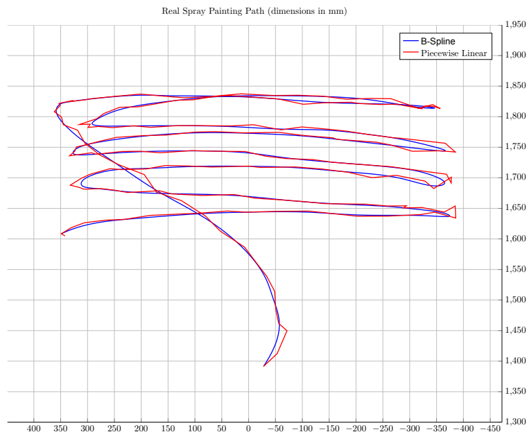
Figure 5.14: B-Spline vs Piecewise Linear X-Y view - Comparison between the B-Spline and the Piecewise Linear Approximation on a portion of the painting path — X-Y plane view
