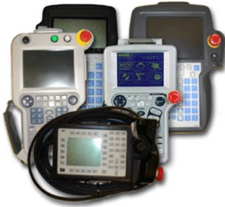
Figure 2.1: Teach Pendants - Each manufacturer has its own layout for the teach pendant
