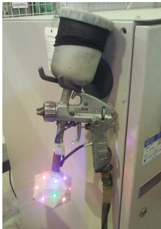
Figure 5.3: Marker Attached to the Industrial Spray Painting Gun - The luminous marker is attached to the bottom side of the spray gun so that it stays clearer from the spraying and the operator's line of sight.
