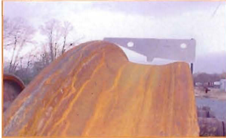
Figure 1.8: Hollow tread and false flange on a train wheel, [8].
