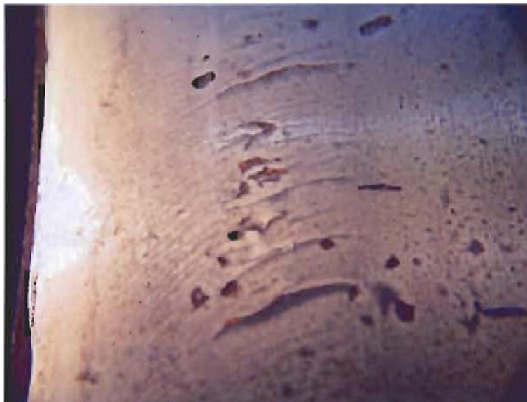
Figure 1.6: Picture of a tread checks, [8].
