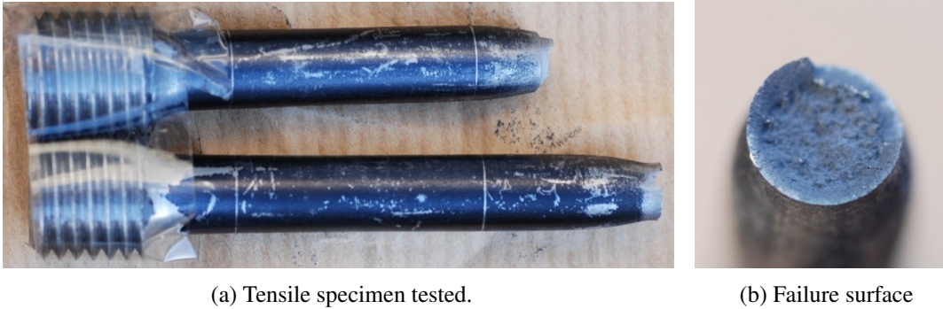
Figure 3.8: Wheel tensile specimen after testing.
