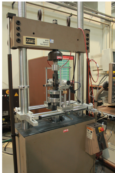
Figure 5.11: MTS® servo-hydraulic machine used to perform the fatigue crack growth tests.
