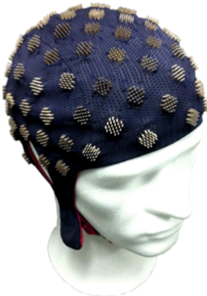
EEG electrode cap composed of 97 individual polyurethane dry multipin electrodes. Copyright: P. Fiedler, TU Ilmenau
