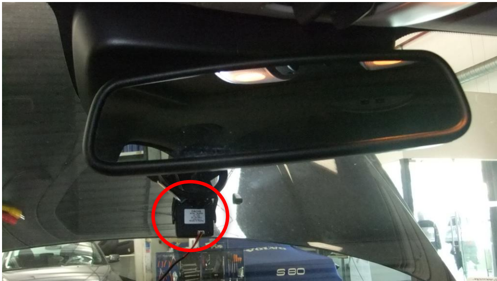
Figure 13 Camera recording the road ahead
