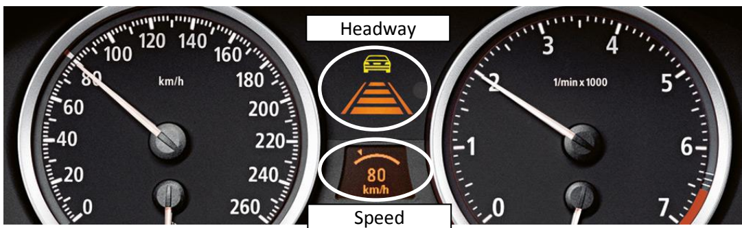
Figure 3 Example of ACC display (BMW)
