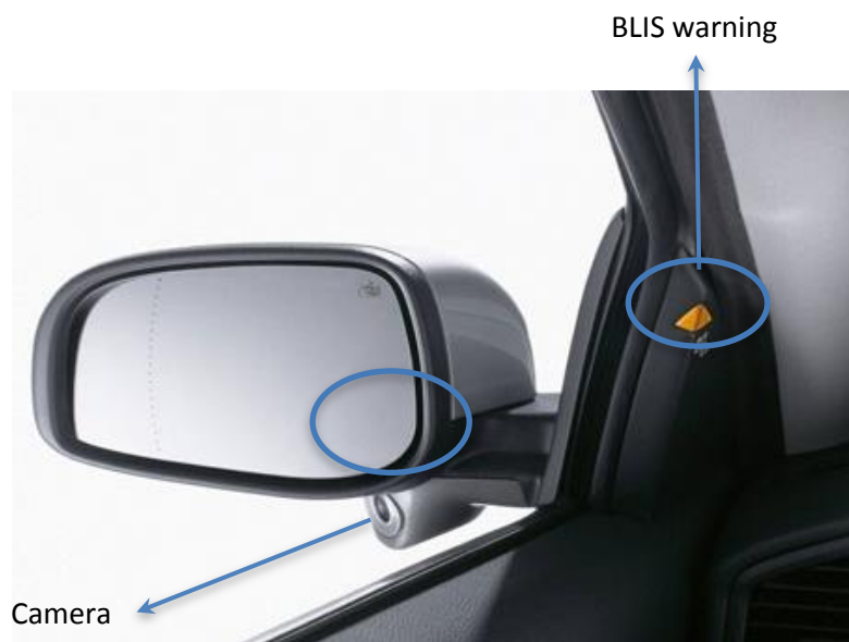
Figure 4 Camera and warning of the Blind Spot Information System (BLIS)
