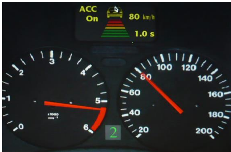
Figure 18 Instrument panel showing information about the ACC functioning
