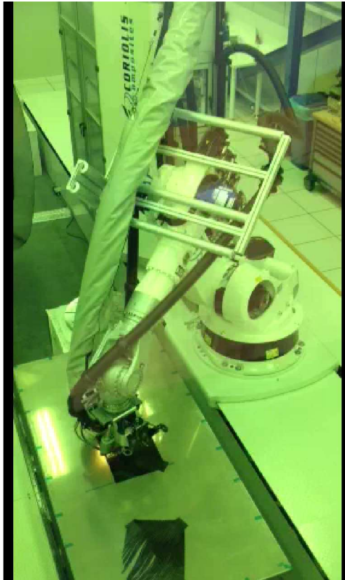
Figure 1.1: Tow-placement machine producing plies with curvilinear fibre path. Courtesy of NLR.
