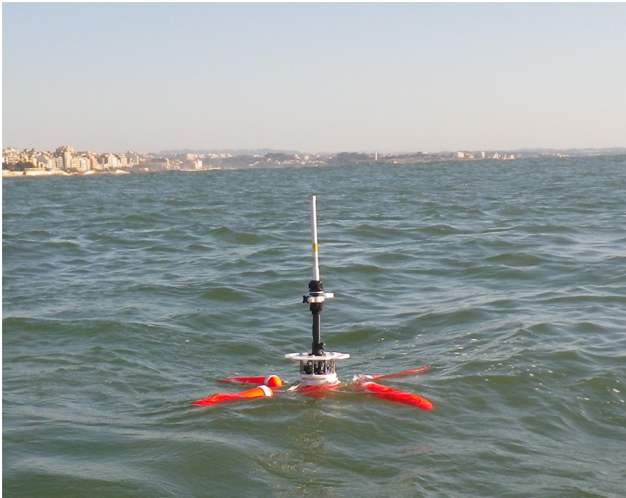
Figure 2.4: The man portable acoustic navigation beacon buoys
