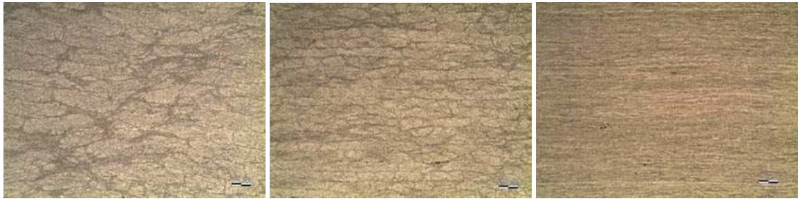
(a) High-grade UD lamina (300 g/m 2 ). (b) Low-grade UD lamina (100 g/m 2 ). (c) Spread-tow UD lamina (30 g/m 2 ).
