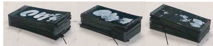
“brush”-like layer splitting shear-driven fibre fracture kink band
