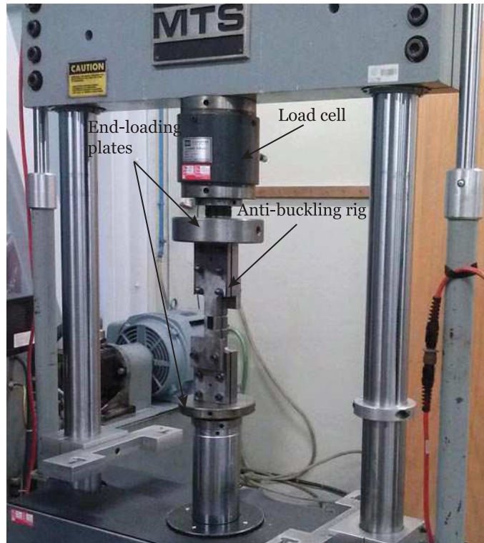
Fig. 5.6. Laminate compressive test setup, with anti-buckling test rig [272].
