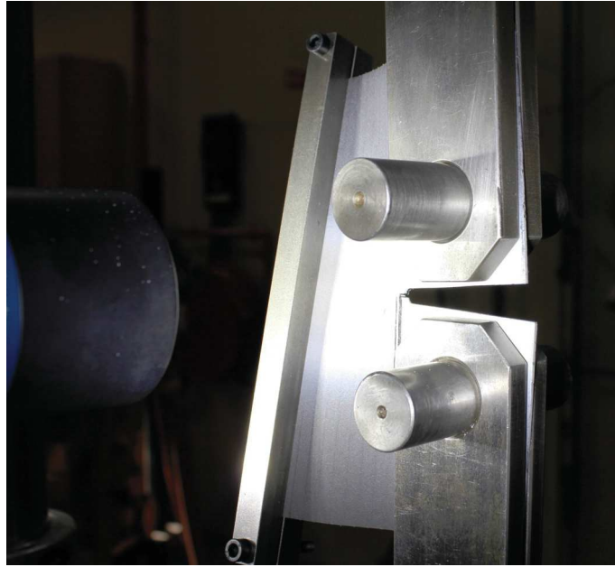
Fig. 10.11. OCT specimen during testing, showing overall buckling of the unnotched end.
