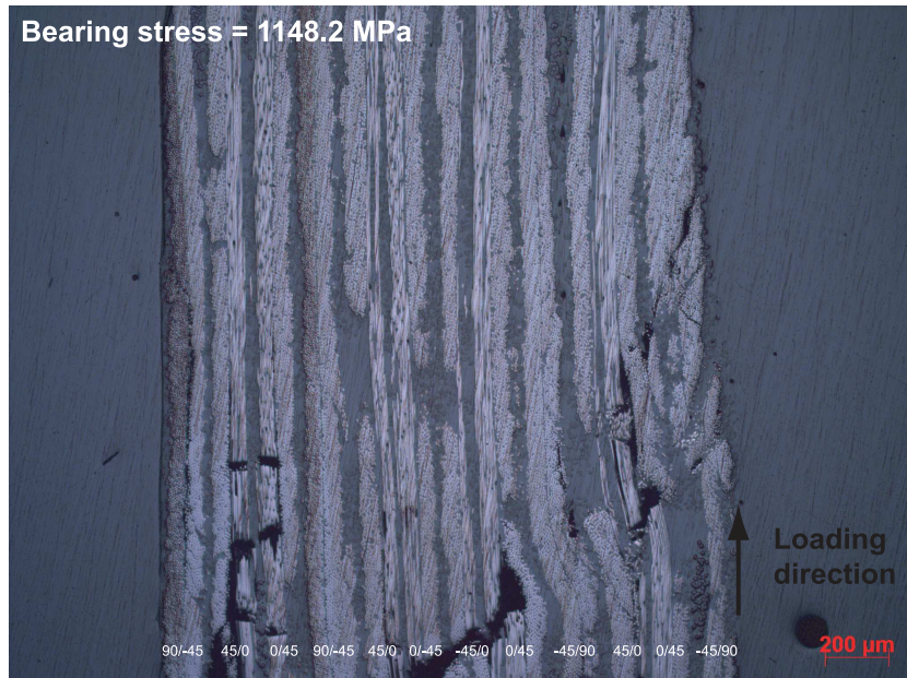
Fig. 5.139. Bearing plane of the blocked laminate at an offset bearing strain of 6% at approximately 1.8 mm from the hole edge. Magnification factor of 5 \times .
