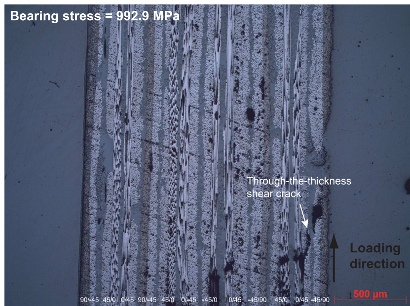
Fig. 5.134. Bearing plane of the blocked laminate at the first load drop at approximately 1.8 mm from the hole edge. Magnification factor of 5×.
