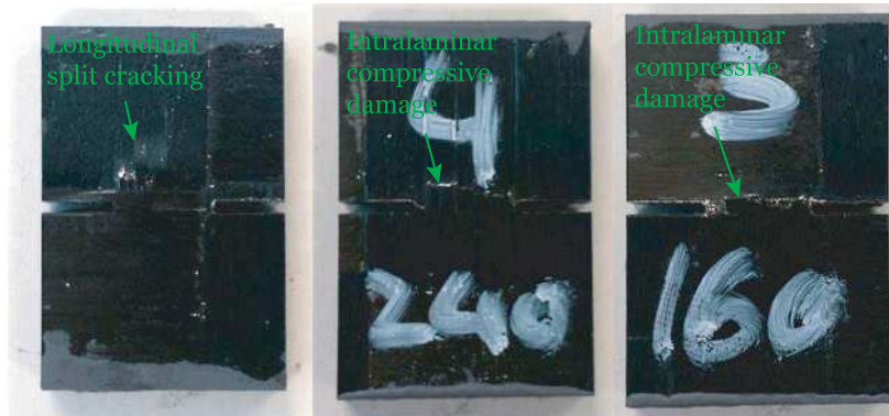
Fig. 4.77. Representative 20 mm wide DENC specimens (geometry C) after testing.
