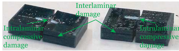
Fig. 4.76. Representative 15 mm wide DENC specimens (geometry B) after testing.
