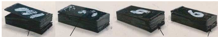
shear-driven fibre fracture kink band “brush”-like layer splitting crushing
