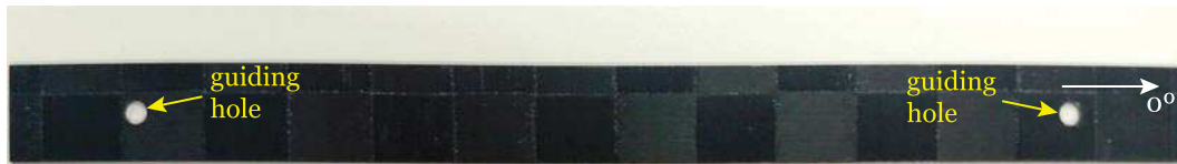
Fig. 4.8. Representative laminate unnotched compression test specimens.
