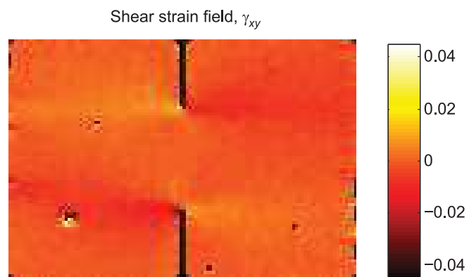
(b) Large DENC test specimen (geometry E) at an applied compressive load of 11.0 kN.
