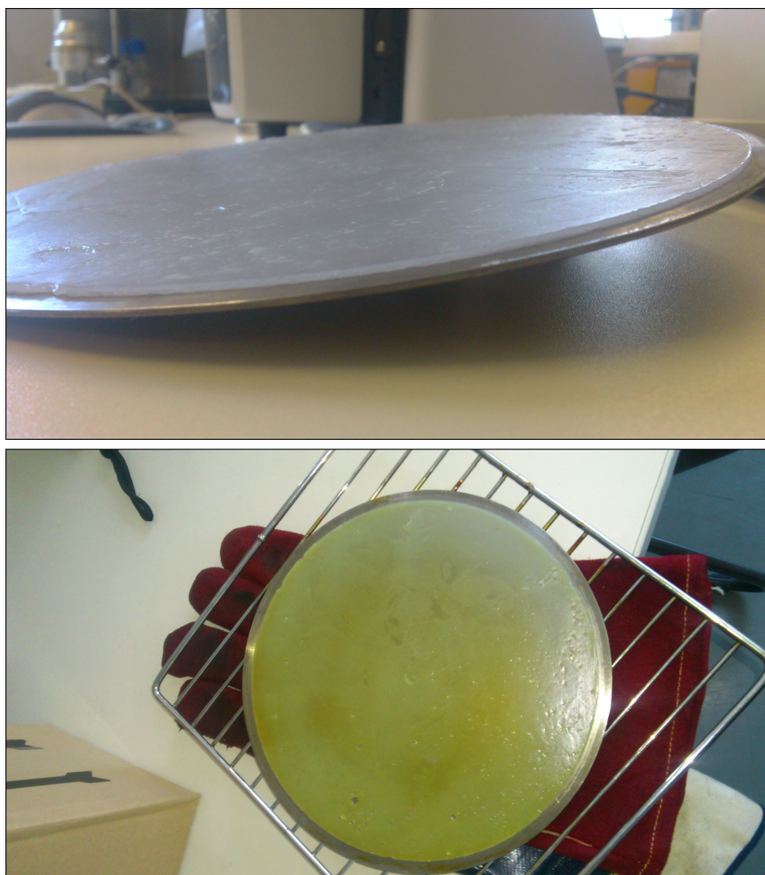
Figure 8.1: Photographs of grease M2, spread across the steel disc with a layer thickness of 1 mm, before and after the aging process.
