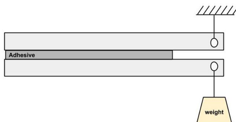
Figure 12: Adhesive joint for creep test
