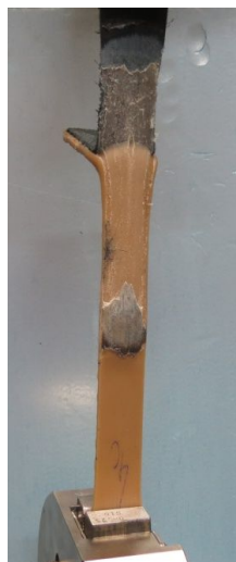
Figure 15 - Specimens leather/TR: with deformation of the TR.
