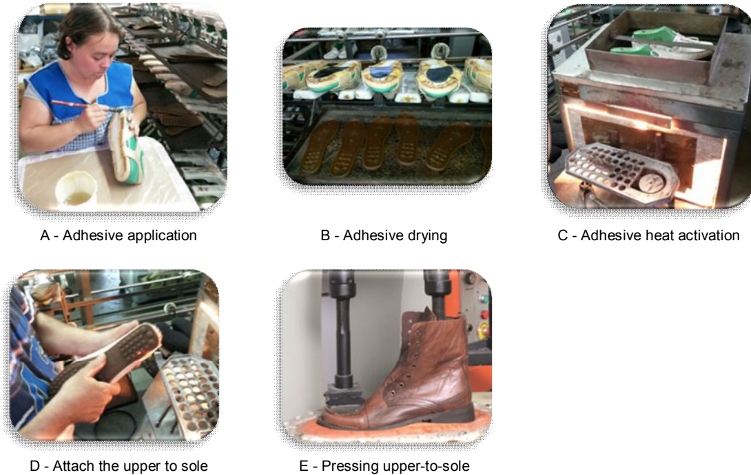
Figure 10: Application of PU adhesive solvent based on assembly step
