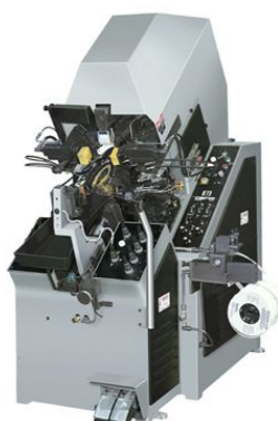
Figure 8: Machine to bond insole to the upper
