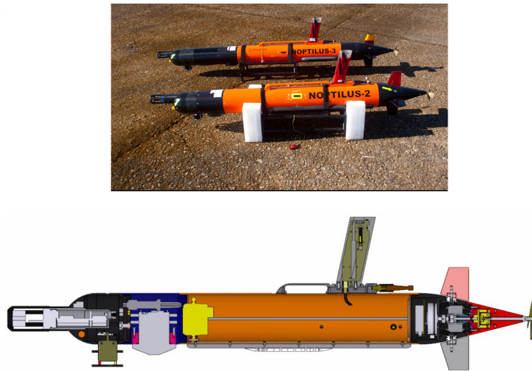
Figure 2.5: LAUV - Light Autonomous Underwater Vehicle
