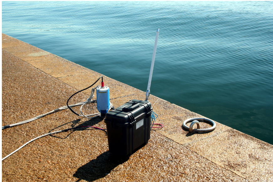
Figure 2.7: Manta communications gateway
