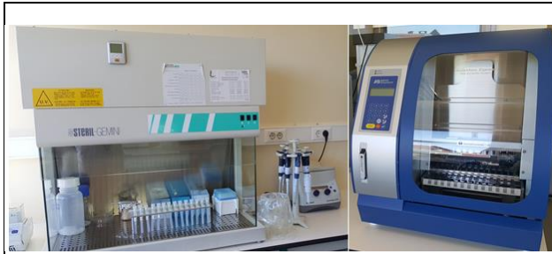
Figure 1 - AutoMate™ Express Instrument and laminar flow camera with pipes support on inside
