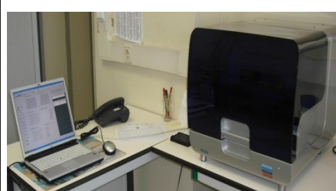
Figure 6 – QIAgility™ robot present in post-PCR room used to prepare the plates for the capillary electrophoresis
