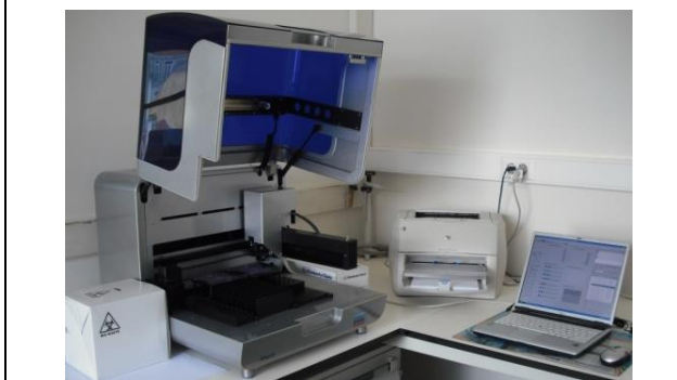
Figure 5 – QIAgility™ robot present in pre-PCR room used to prepare the plates for DNA quantification
