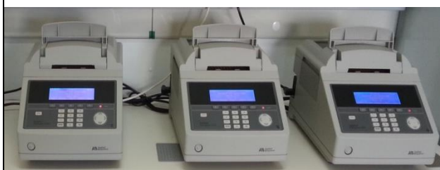
Figure 3 – Thermal cycler GeneAmp® PCR System 9700 with gold-plated silver 96-Well Block equipment
