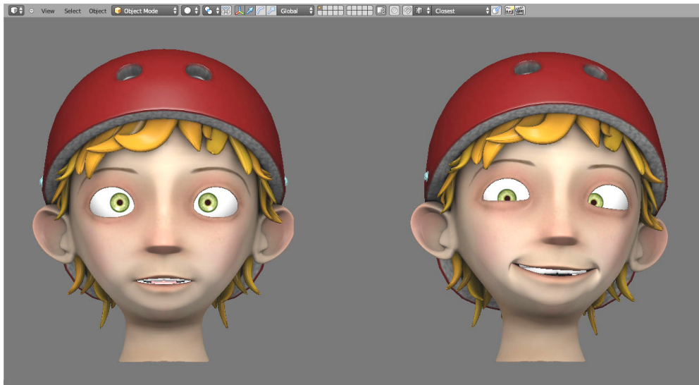
Figure 2.12: Examples of blendshapes for the face of the character Nene in Blender; left: a neutral pose to represent an idle state for the character as a starting point for both rig and animation debugging; right: a blendshape pose sculpted to simulate a smile (facial model is copyright of FaceInMotion).
