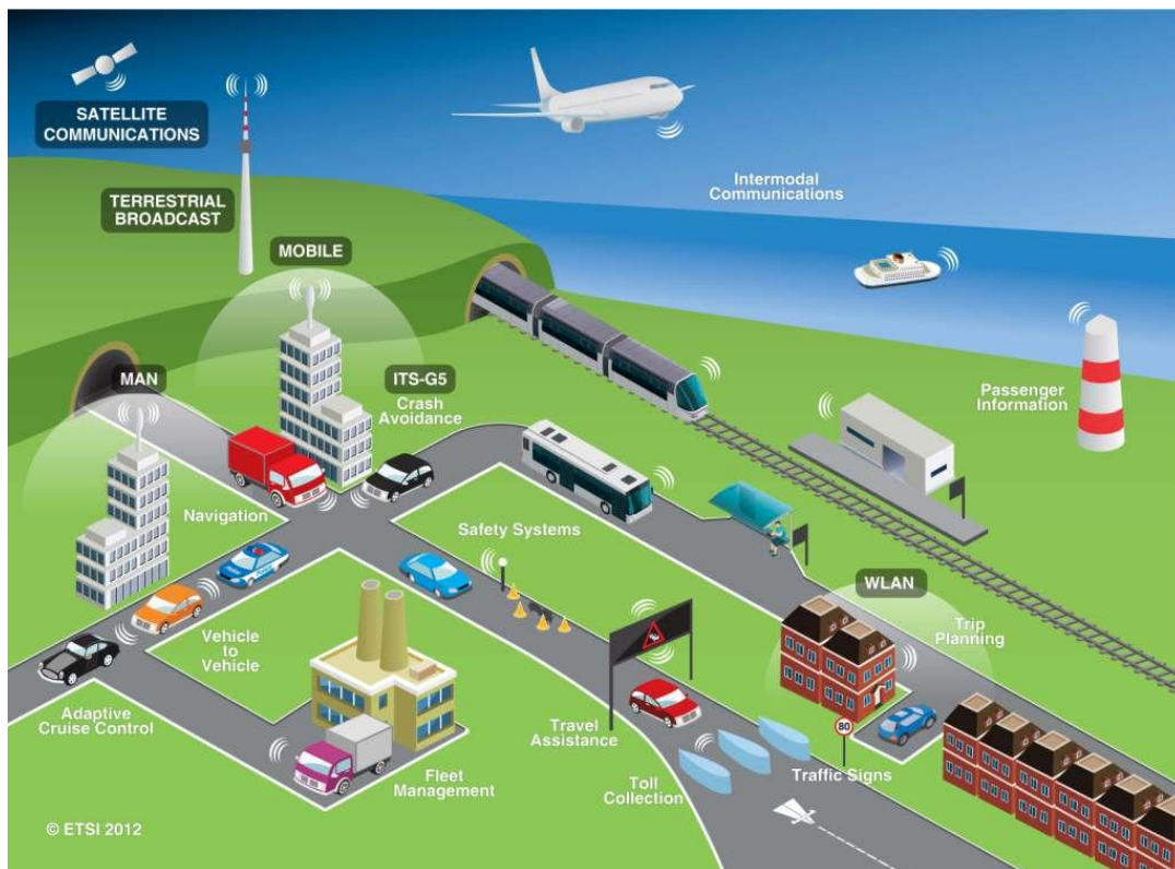
Figure 1.3: Intelligent Transportation Systems use cases and potential communication technologies, defined by ETSI ITS
