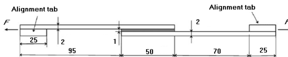
Figure 9 – Geometry of the SLJ test specimens (dimensions in mm).
