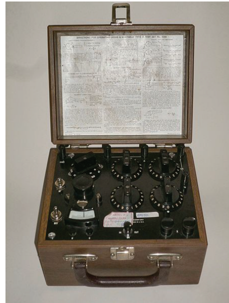
(b) Leeds & Northrup instrument used for bridge circuit tests in early XX century.
