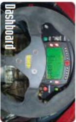
The AIM dashboard developed expressly by Gian supplies the driver with the lap time, RPM, speed, gear, water temperature, oil temperature and pressure, oil downshifts on your PC, for the 2005 model part or complete data recording of accelerometer, steering and steering in kilometers.
