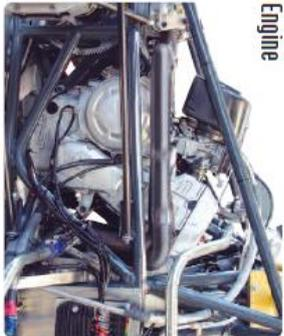
Yamaha Fazer 1000 cc, 4 cylinders with 4 stroke cycles, 5 valves per cylinder, 2 overhead camshafts with distributor chain. Cooling guaranteed by water and oil radiators, 4 carburetors.
