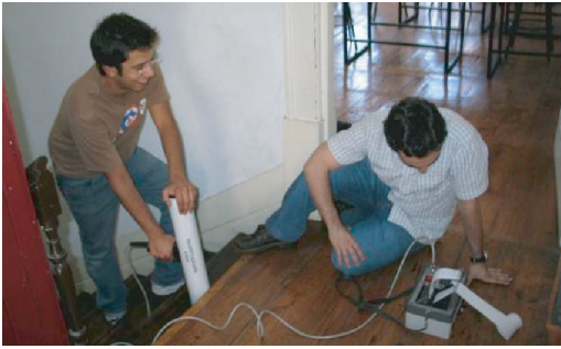
Figure 9. Use of the resistograph on wood stairs. São Domingos building. XIX century (1856), Porto.
