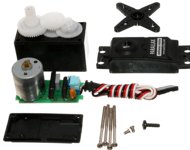
Figure 1.1: RC Servo disassembled showing its main elements [1]
