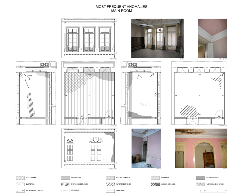
Figure 3. Plans, of floor and ceiling, and elevations of a main interior space of a bourgeois house in Porto, to scale 1:20, indicating the most frequent anomalies.
