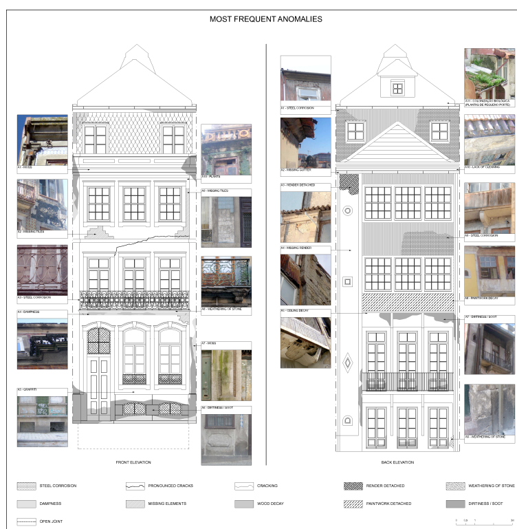
Figure 2. Elevations, of street and courtyard, to scale 1:50, of a bourgeois house in Porto. Model, corresponding to the Liberal period, indicating the most frequent anomalies.
