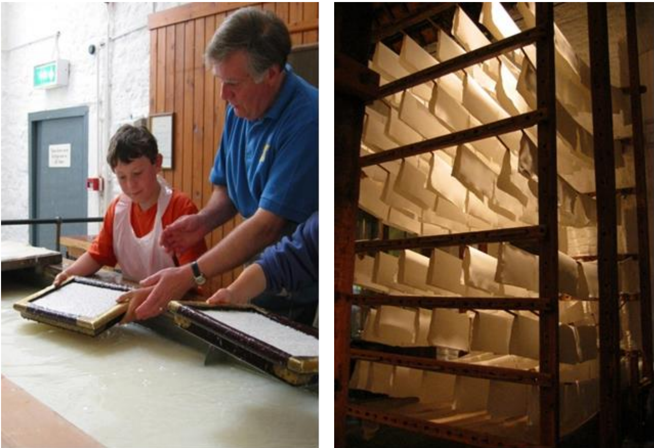
Figure 109 - Wookey Hole Paper Mill, UK. (Left) Vat-man teaching a child to form a sheet of handmade paper; (Right) handmade paper drying in the racks. Images in the public domain.
