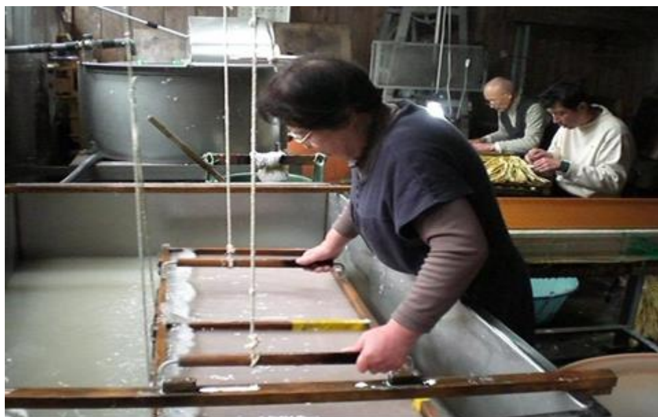
Figure 108 - Making a sheet of washi , (two men cleaning bast fibres by hand can be seen in the background). Photograph by Rina Aoki. Courtesy of the Echizen Washi Village, Echizen, Japan.
