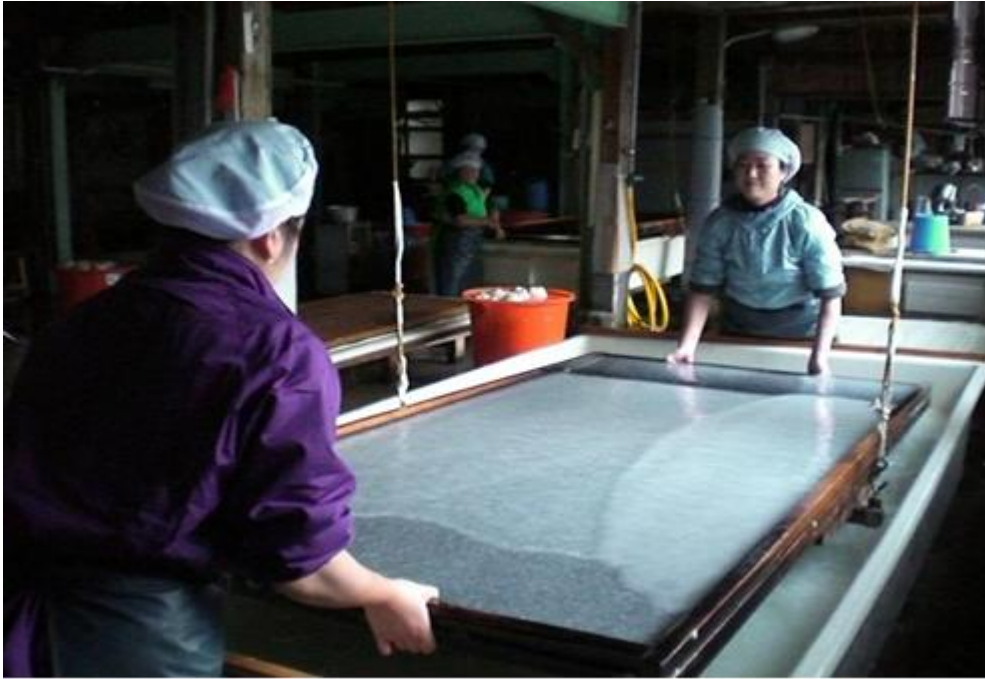
Figure 115 - Contemporary washi makers forming an extra-large sheet. Photo by Rina Aoki with permission from the Echizen Washi Village, Echizen, Japan.
