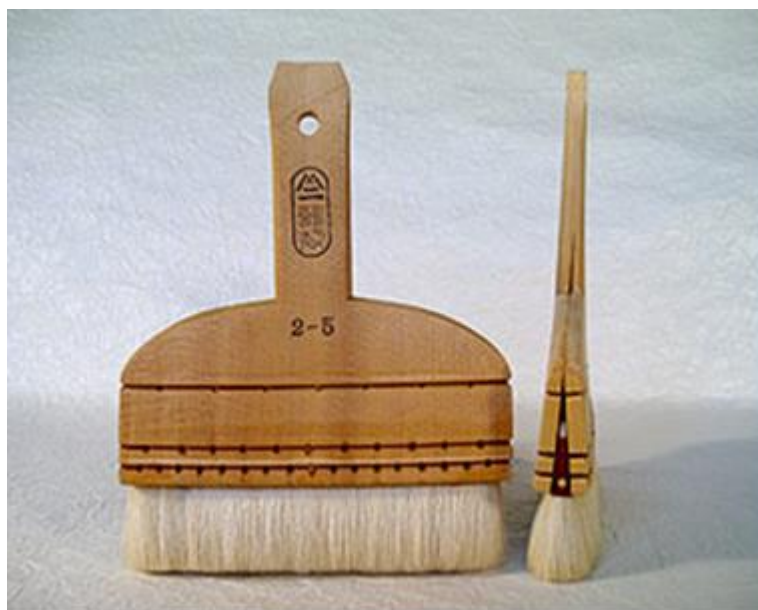
Figure 123 - Noribake Japanese brushes for pasting or painting, made in the traditional way with cherry wood and white sheep hair. Image courtesy of The Japanese Paper Place © 2011.
