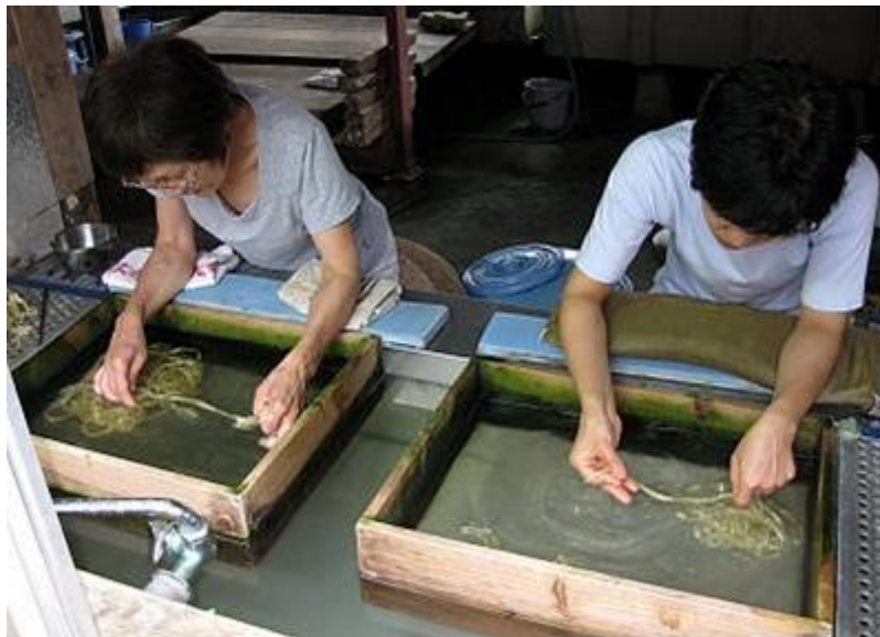
Figure 106 - Removing particles from kozo fibres by hand. Image © Agency for Cultural Affairs, UNESCO.
