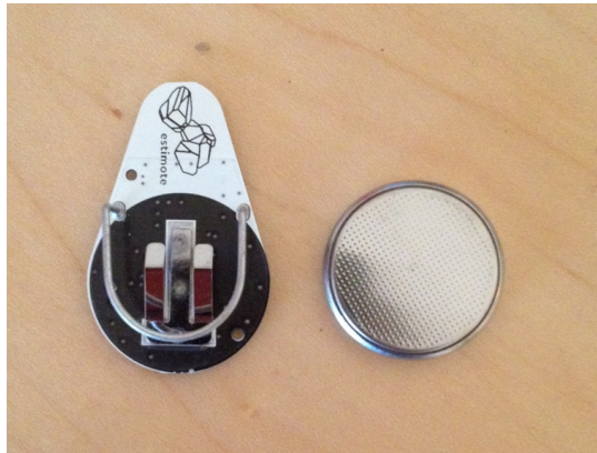
Figure 38 - Estimote beacons' hardware [182] The beacon hardware, with battery unattached.
