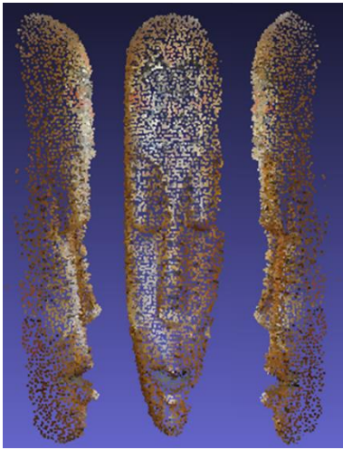
Figure 21: Three views of 5 aligned point clouds of a small object.
