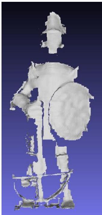
Figure 41: 3D model reconstruction with David laserscanner.
