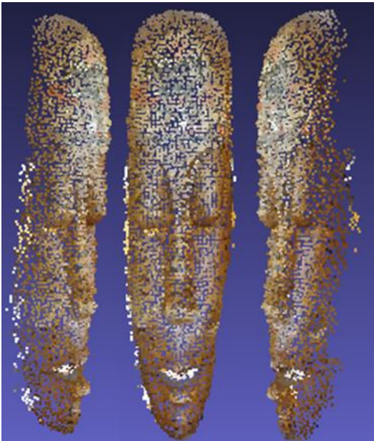
Figure 39: 3D model reconstruction with Microsoft Kinect.
