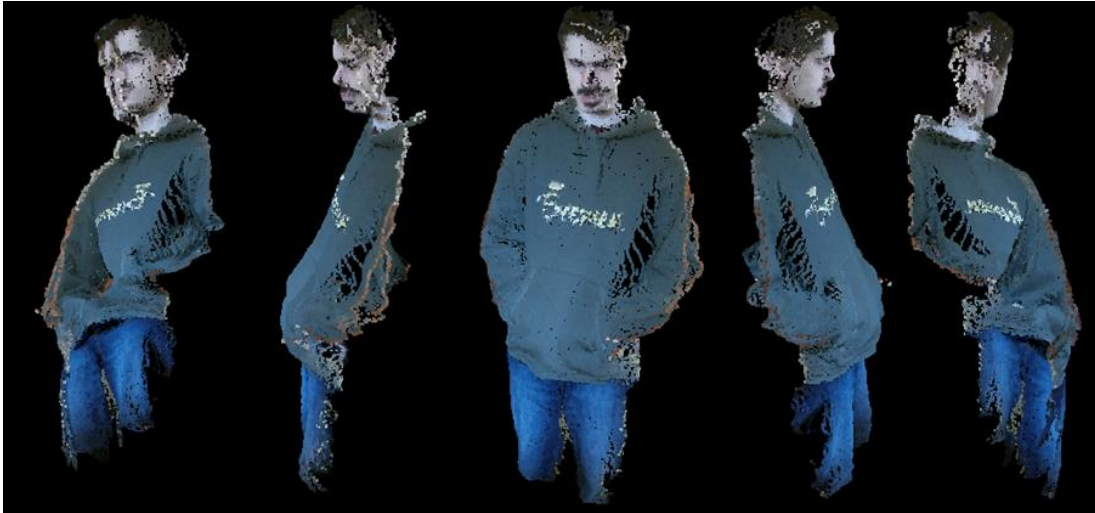
Figure 27: Multiple views of the result of rigid registration between two point clouds with small deformations.
