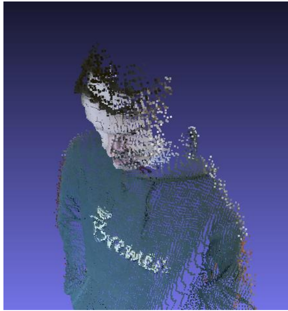
Figure 43: Rigid registration of two point clouds with deformations.
