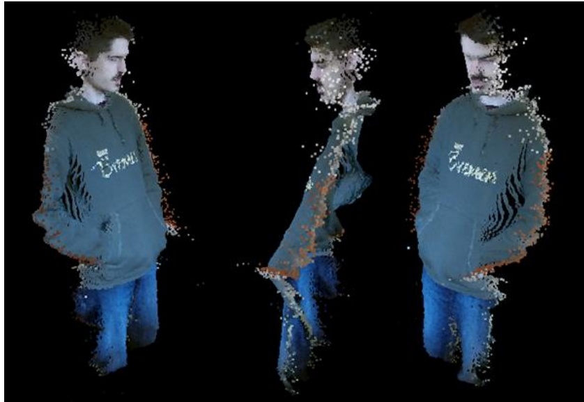
Figure 15: Example of a point cloud before the noise reduction algorithm.
