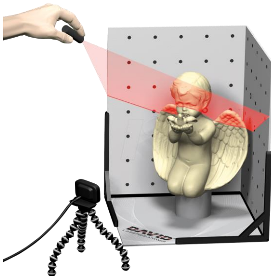
Figure 36: Illustration of the use of the David laserscanner.
