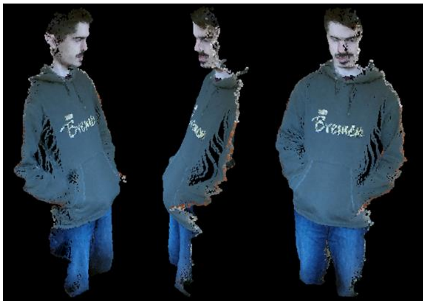
Figure 16: The same point cloud of Figure 6 after the noise reduction algorithm.
