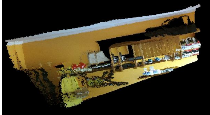
Figure 19: Example of failed registration when the sensor is moving parallel to a surface with big flat regions.
