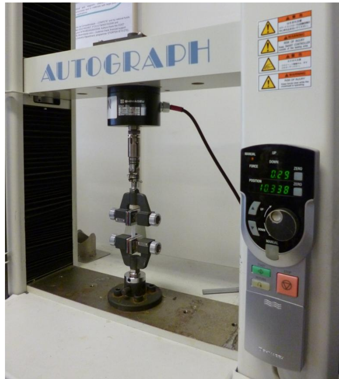
Figure 9 - Chitosan-GPTMS membrane assembled in the universal testing machine.
