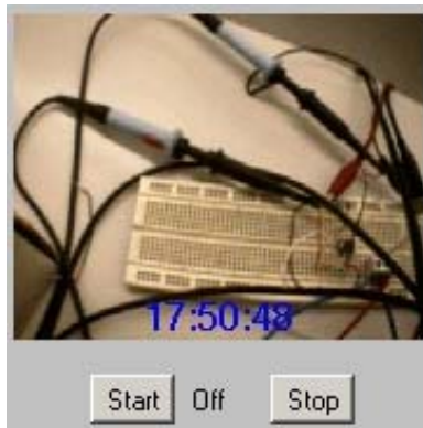
Fig. 3. Image of the circuit under test from one of the Web cams installed at the REW. The interface has start / stop buttons that allow reducing the bandwidth requirements for certain periods, while using the real-time clock as an indicator of the current status.
