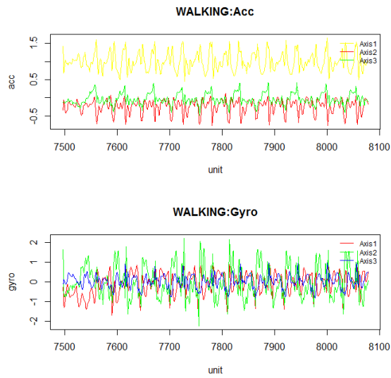
Figure A.10: Plot of the sensor data which represents the activity "Walking".
