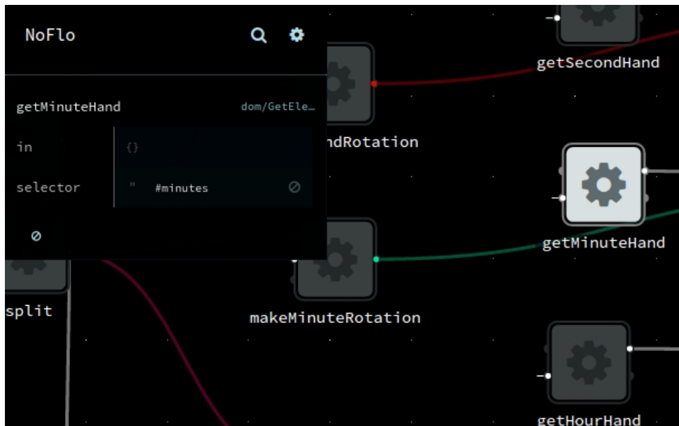
Figure 2.5: Example of node expansion in NoFlo [Ber]
