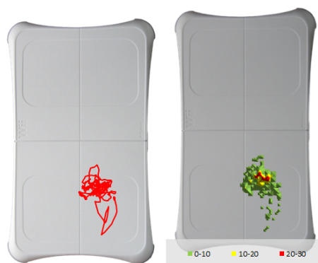
Figure A.4: Participant 4 COP's path (left) and frequency map (right) while playing Scooter Chase on test phase 1.
