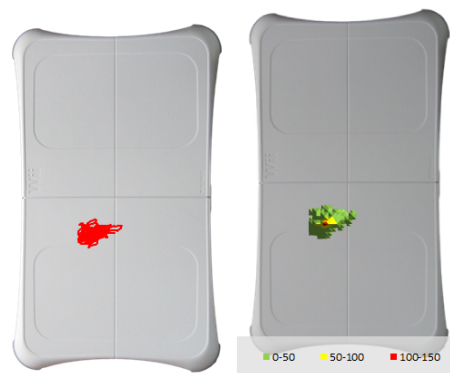
Figure A.6: Participant 6 COP's path (left) and frequency map (right) while playing Scooter Chase on test phase 1.
