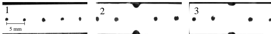
Fig 5. Smooth cylindrical specimen (1) and notched cylindrical specimens with high (2) and low (3) notch severity.
